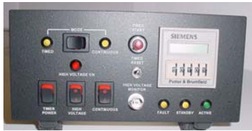
Stand-alone Timer (part #490-0212) System operation with programmable cure control
